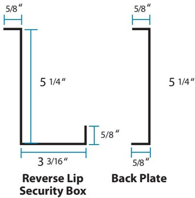
Security Box to be 24 gauge galvanized steel unless specified.
