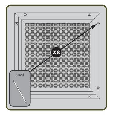
2 Use the appropriate drill bit to drill 8 holes on the previously marked location.
