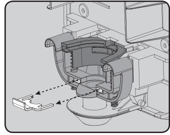
**STEP 2:** Product is designed to accept GOJO®1250 mL soap refills. With the bottle inverted as shown, depress Soap Bottle Nipple upward.
