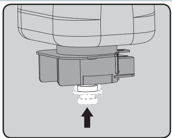
**STEP 3:** Align Soap Bottle Bracket with slots in Receiver (Blue) (2) and insert. Keeping bottle vertical and allowing Nipple (1) to drop into hole.
