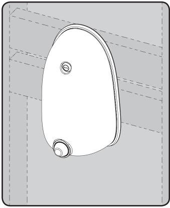
2 Open the unit using the Key provided and the front cover will rotate downward.
