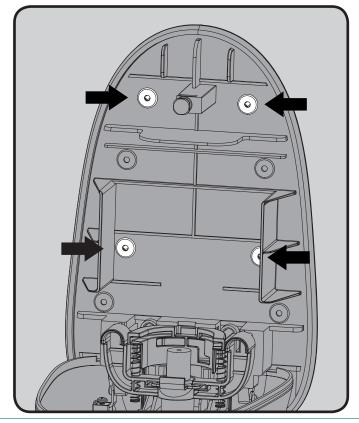
4 Install supplied Mounting Hardware through the four (4) mounting locations using the supplied Torx driver to secure into brace (supplied by installer) or into wall structure.
