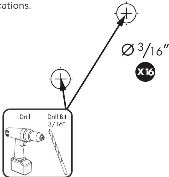
3. Use the driver bit and the mounting hardware provided to mount the mirror securely and tightly against the mounting surface. Ensure the mounting structure and mounting hardware can safely support the product in use. If mounting on drywall and not to stud, use the appropriate anchors and fasteners for application. (Recommend screw in EZ anchor or equal for drywall.)
