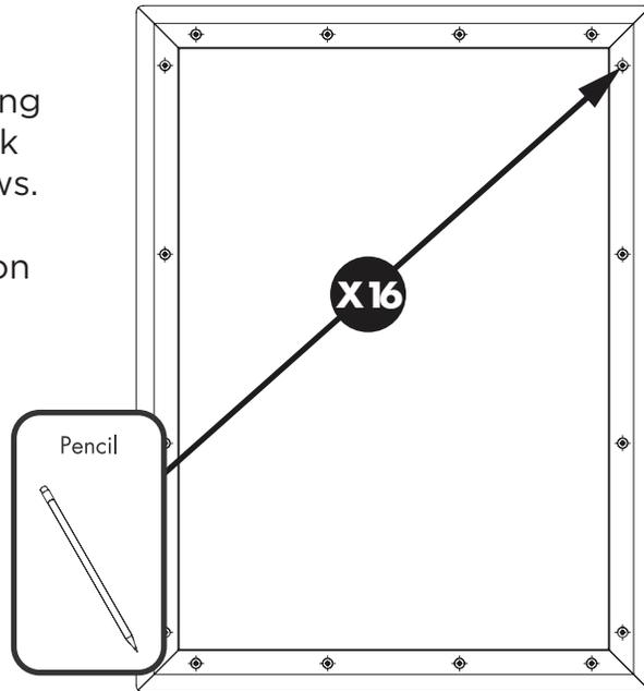
2. Use the appropriate drill bit to drill 16 holes in the previously marked locations.
