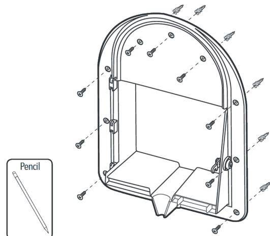
3. Remove the dispenser from the wall and drill the 9 marked Drill holes using a 1/8" (3mm) drill.
