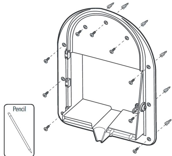
4. Remove the dispenser from the wall and drill ALL the marked holes using a 1/8" (3mm) drill, centered as closely as possible into the markings.
