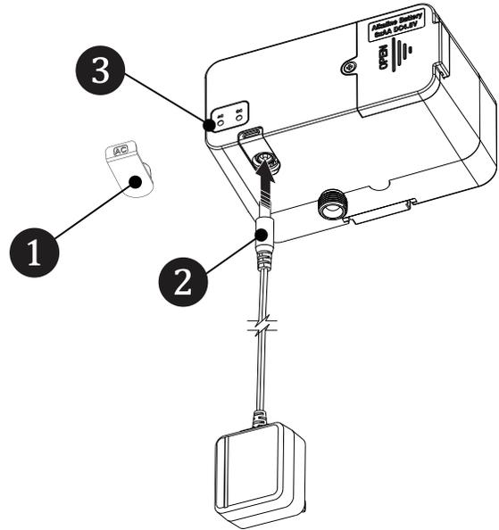
2. If you are currently using batteries in your faucet and wish to change to A/C power, remove batteries from enclosure as shown before plugging in the adapter.
