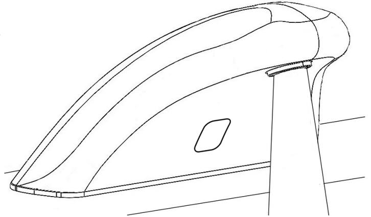
2. Remove, clean and reinstall the vandal-resistant laminar flow outlet to the faucet using the included aerator wrench.
