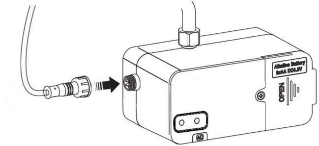
12. After securing the hoses and electrical connections, align the solenoid assembly and slide it over the mounting bracket on the wall.
