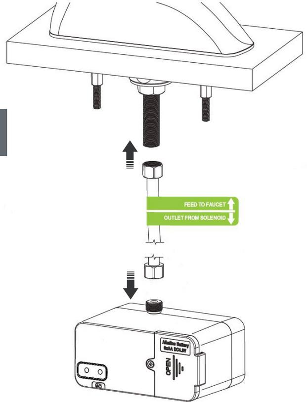
10. Connect the under counter mixer (UCM), to the bottom of the solenoid box. Next make the water connections between the shut off valves and the solenoid assembly using 3/8" compression style hoses (*not included* ).
