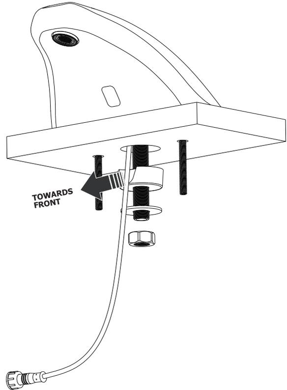
5. From under the sink, install the “U” washers **1** onto the threaded mounting posts and secure with the mounting nuts **2**. Ensure that the “U” washers are perpendicular to the wall surface for added leverage and wrench-tighten.
