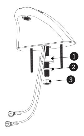
3. Insert the sensor wires, faucet shank and threaded mounting Posts 1 through the holes of the basin. Take extra precautions to avoid pinching any wires. Once the faucet is positioned, verify that the rear of faucet is properly resting on the rubber base gasket and does not overlap the rubber base gasket.
