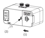
Step 3: Put the battery holder back into the solenoid housing and push the battery box cover to the left and then lock the cover with the screw.
