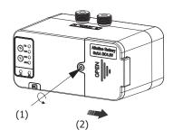
Step 1: Loosen the screw and push the battery box cover to the right to open.
