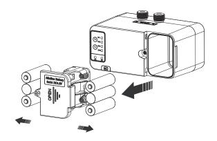
Step 2: Remove the batteries.
