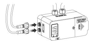
13. After securing the hoses and electrical connections, align the solenoid assembly and slide it over the mounting bracket on the wall.
