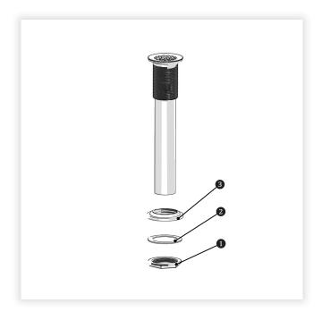
2. Apply included Upper Drain Seal (1) or Plumber's Putty to the underside of the Upper Flange. Insert Drain Assembly into drain hole of sink from above.
