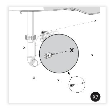
4. Re-install the Trap Cover under the Sink. Use the supplied #10-24 x 0.5" Screws to fasten the cover to the Sink using the supplied T25 Security Torx Driver (X5).
