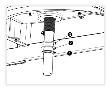
4. Assemble all remaining drain connections (not included) and hand tighten only at this time.
