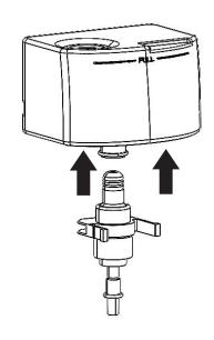
Reinstall the pump/reservoir assembly back into the dispenser by lifting the pump nozzle up while inserting the assembly into the dispenser.
