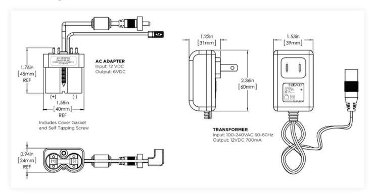
If you wish to change your faucet from battery power to AC power, remove battery power module cover and batteries. Replace with AC Adapter and secure with Phillips head screw. Secure included Grounding Lug between existing screw and Metal Bracket of Solenoid. Connect Grouding Wire to Grounding Lug. Connect AC Power Module to AC Transformer.
