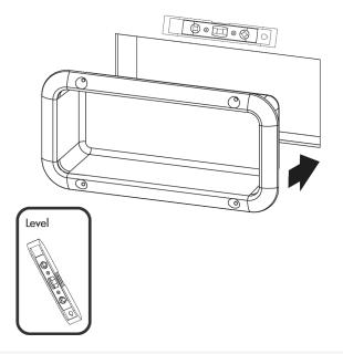
3. Install supplied Mounting Hardware through the four (4) mounting locations using the supplied Torx Bit tool into a secure brace (supplied by installer) or into wall. This will support the Ligature Resistant Recessed shelf. Ensure the mounting structure and mounting hardware can safely support the product in use.
