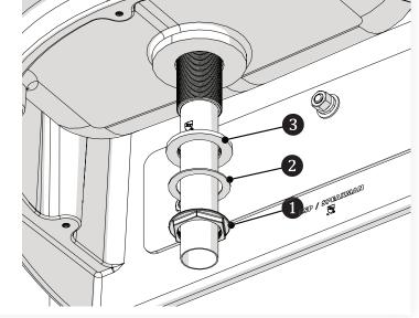
4. Assemble all remaining drain connections (not included) and hand tighten only at this time.
