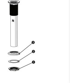
2. Apply included Upper Drain Seal (1) or Plumber's Putty to the underside of the Upper Flange. Insert Drain Assembly into drain hole of sink from above.
