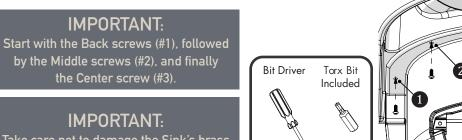
Take care not to damage the Sink's brass inserts. Limit torque to 20 in\*lbs.
