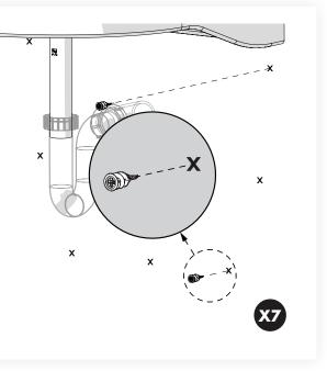
4. Re-install the Trap Cover under the Sink. Use the supplied #10-24 x 0.5" Screws to fasten the cover to the Sink using the supplied T25 Security Torx Driver (X5).
