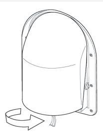
6. Lock the dispenser using the key. Remove first towel to check proper feed.
