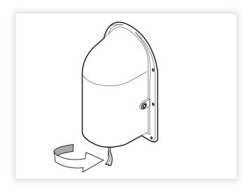
6. Lock the dispenser using the key. Remove first paper towel to check proper feed.
