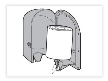
5. Push the roll into the door and close the cover. Check to ensure paper towel is not pinched between cover and base.
