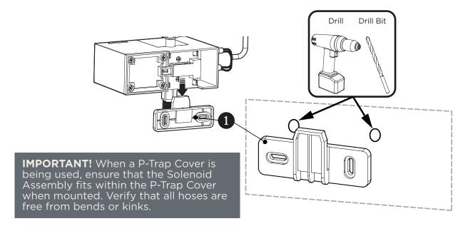
12. After securing the Bracket to the mounting surface, align and slide Solenoid Assembly over Mounting Bracket.
