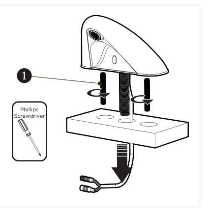
3. From beneath, install Rubber Wire Guard (1) (with notch facing towards rear) over the shank and pass the Sensor wires through the notch to prevent pinching of wires. Install Metal Washer (2) and Mounting Nut (3) onto shank. Hold Faucet in position and wrench tighten Mounting Nut (3). Verify that Sensor wires are not pinched.
