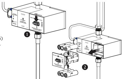
15. Reinstall the Battery Enclosure to the Solenoid Body (1). Make sure to press the indicated location until the battery door is fully seated and locks into position (2).
