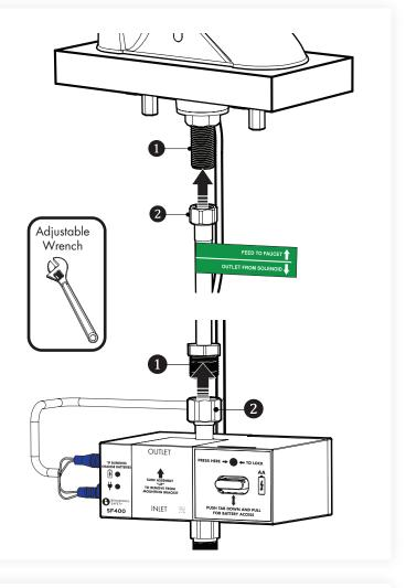
8. Place the Solenoid Assembly against the desired mounting surface while ensuring adequate clearance for servicing of all connections. If using the optional A/C Adapter (not supplied), consider the distance to the nearest electrical outlet. Solenoid Assembly should be mounted so the inlet and outlet ports are aligned vertically. Mark location of Solenoid Assembly on the mounting surface using a pencil.
