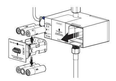
2. Reinstall the Battery Enclosure to the Solenoid Body (1). Connect the A/C Adapter to the Solenoid Body (2). Plug the A/C Adapter into the wall outlet. The A/C light (3) should illuminate.
