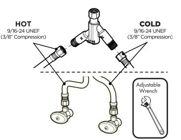
10. Thread the Under Counter Mixer (UCM) to the male connection of the 12in flex hose (marked with Yellow label). Position inlets of UCM so they are accessible. Connect remaining end of YELLOW labeled hose to the Inlet of the Solenoid. Wrench tighten connections. Take care to not over tighten connections or damage may occur.
