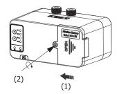
Step 4: Open the AC adapter cover on the solenoid body (1) (Shown separated for clarity). Connect the A/C Adapter to the solenoid body (2). Plug the A/C Adapter into the wall outlet. The A/C light (3) will illuminate.
