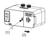
Step 2: Remove the batteries.
