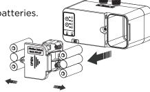
Step 3: Put the battery holder back into the solenoid housing and push the battery box cover to the left and then lock the cover with the screw.
